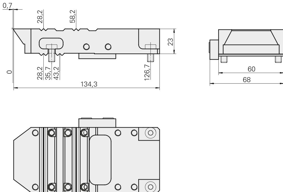
**Distance plate INDEX MS24-6****X direction, for use of tool drive unit VDI shank****Offset dimensions**
