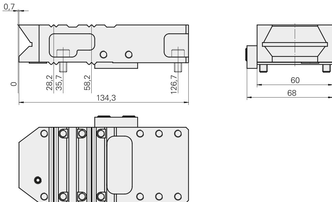
**Distance plate INDEX MS24-6****Z direction, for use of tool holders with slide system MS16/MS22**
