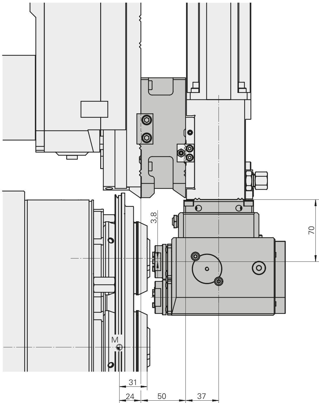
**Tool drive unit INDEX MS24-6****Setup option on cross slide units 1.1 - 6.2****Installation example****VDI shank straight, axis-offset, tool drive unit offset back in X direction**
