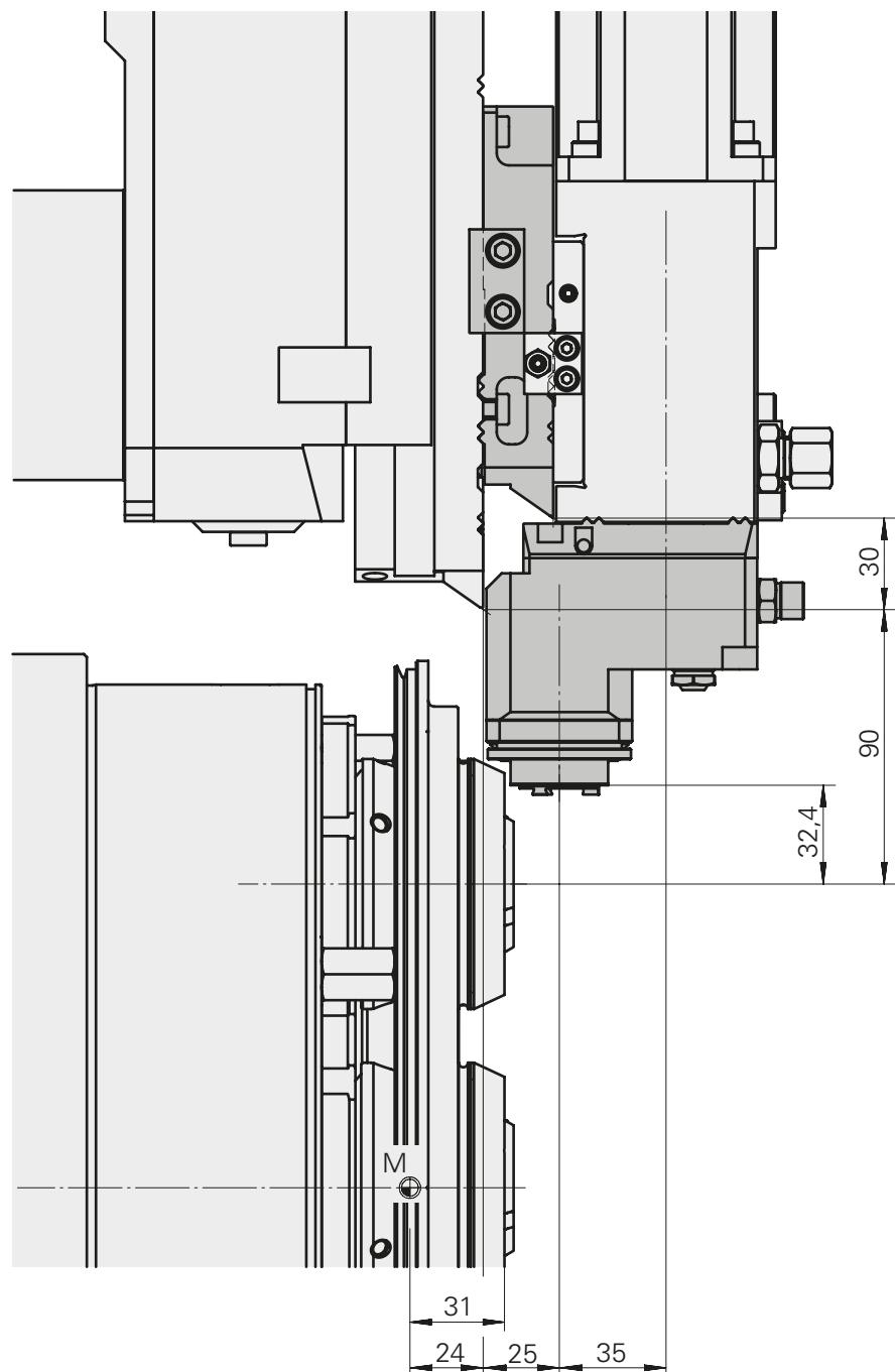
**Distance plate INDEX MS24-6****Z direction, for use of tool holders with W-serration fixation**
