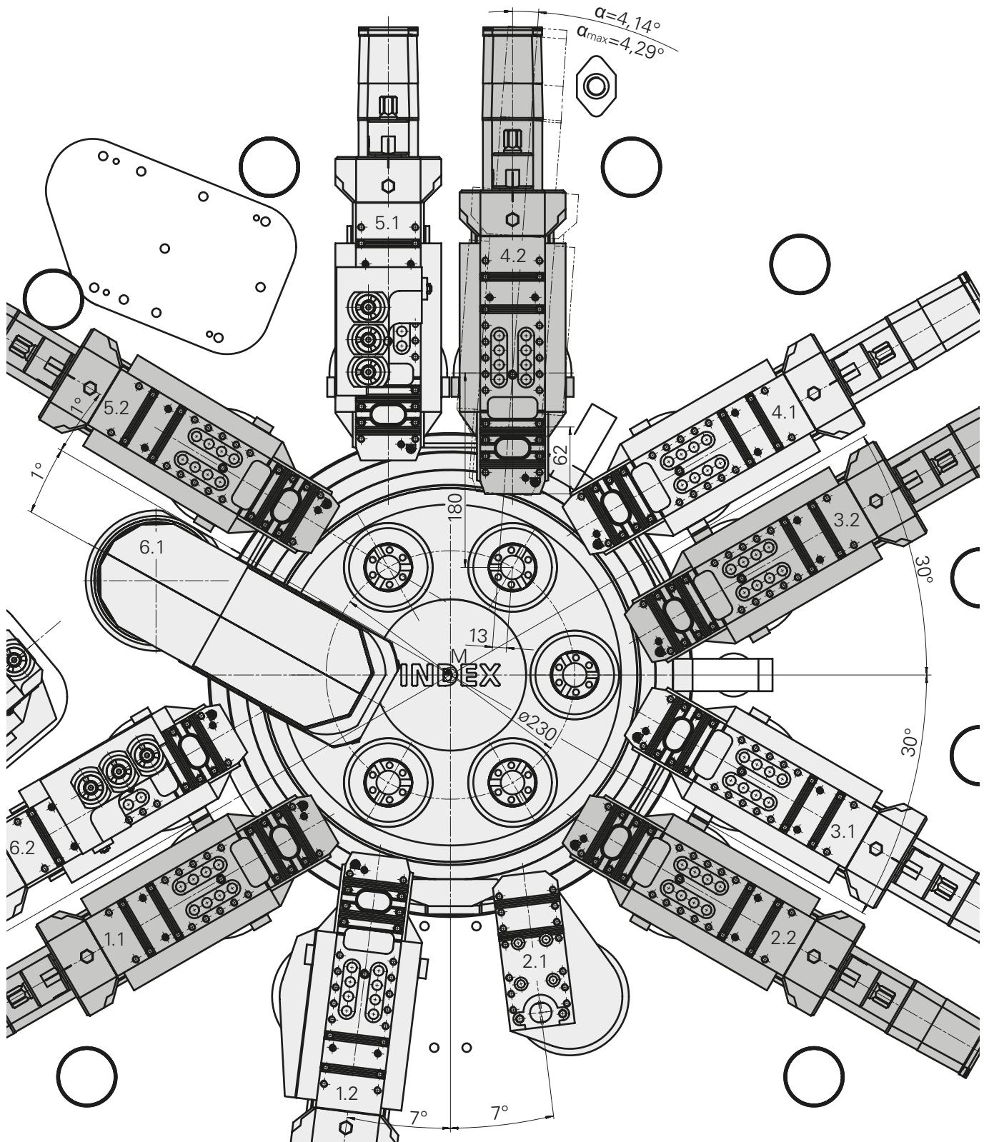
**Tool drive unit INDEX MS24-6****Setup option on cross slide units 1.1 - 6.2****Installation example****VDI shank angled, tool drive unit offset in Z direction**
