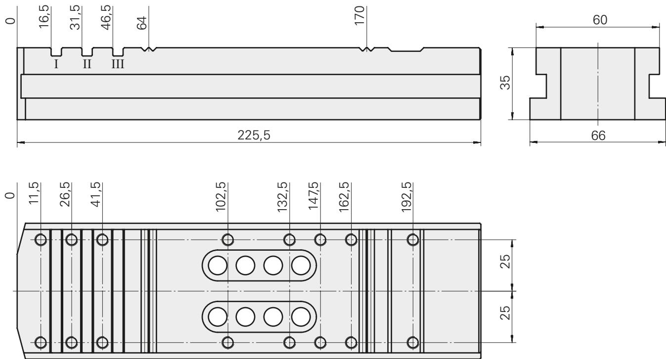
**Modular design of INDEX MS24-6****Base holder with drill holder D20mm/D28.5mm****Cross slide unit 1.2, 2.1, 3.2, 4.1, 5.2, machining in X direction**
