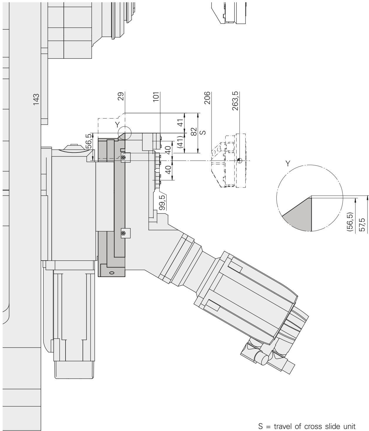
**Synchronized spindle INDEX MS40-8****Rear end machining on swivel axis 7.2, 8.1**
