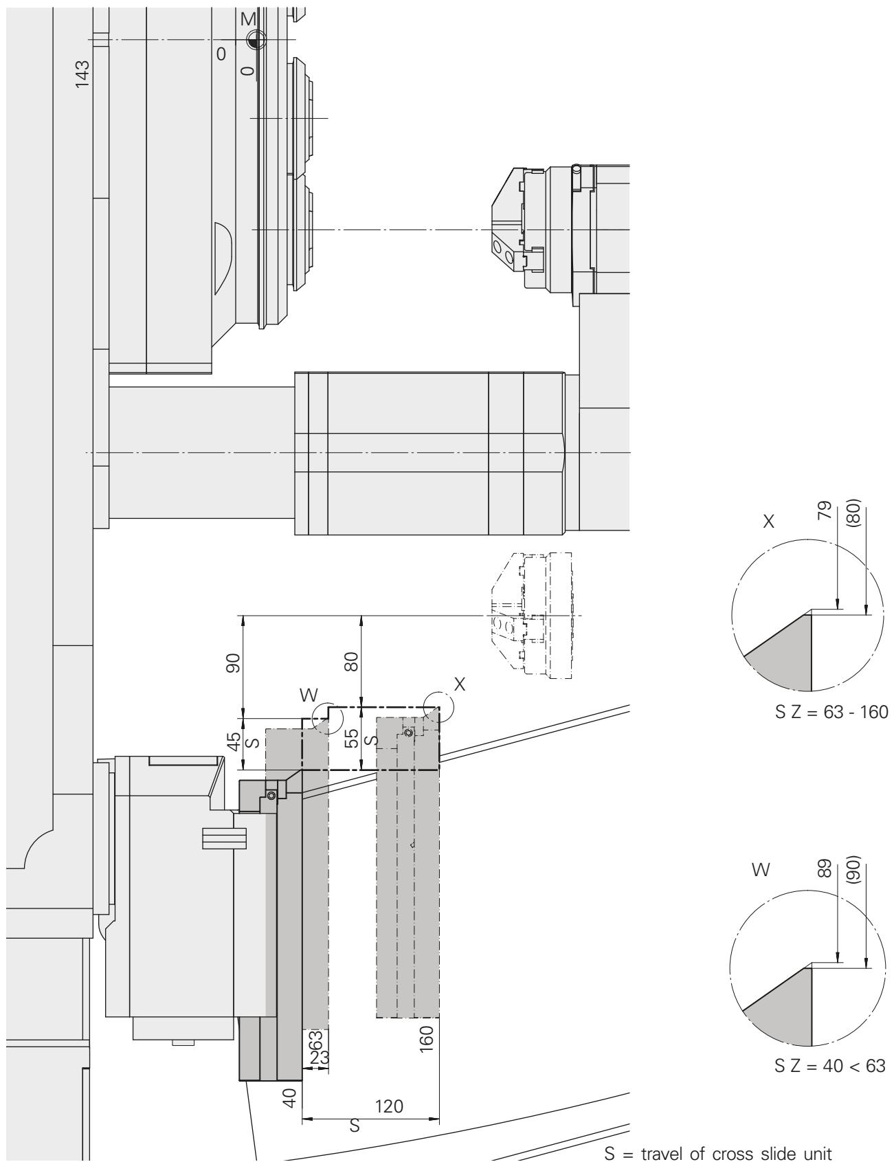
**Travel of cross slide unit INDEX MS40-8****Cross slide unit X-NC / Z rigid 7.3/8.3**
