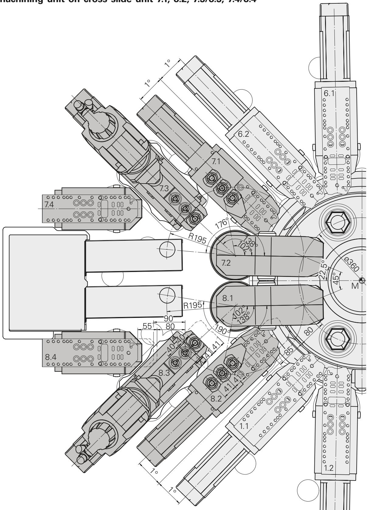
**Y axis INDEX MS40-8****Attachable to cross slide unit 3.1, 4.1, 5.1, 6.1, 7.2**
