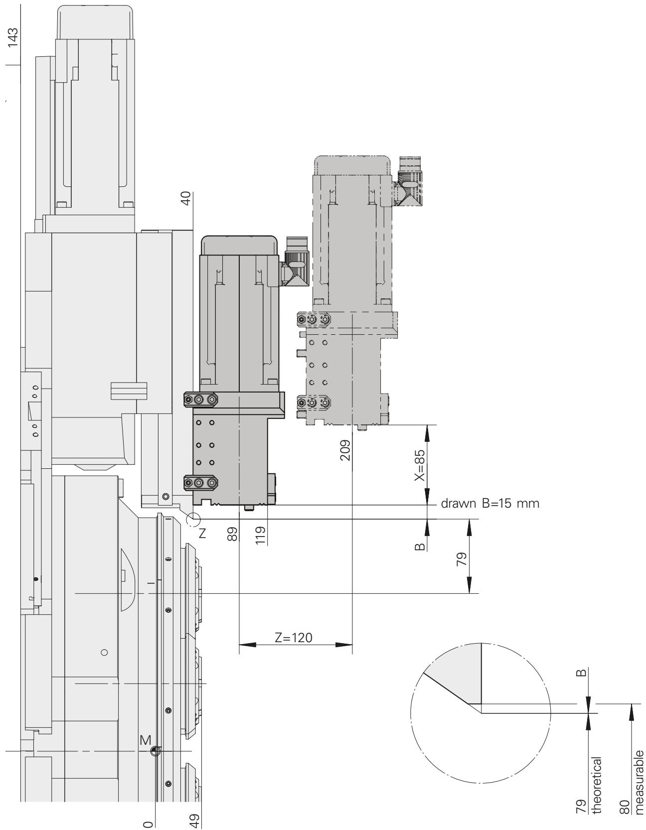
**Tool drive unit shank VDI25, INDEX MS40-8****Cross slide unit 1.1 - 8.2****Oil drain**
