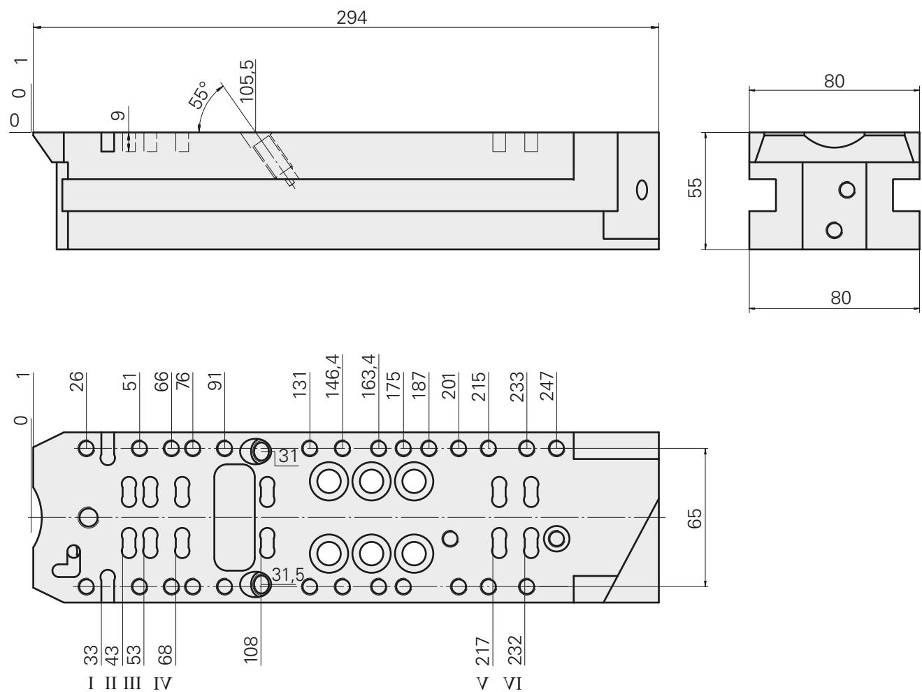
**Modular design of INDEX MS40-8****Grooving tool holder****Cross slide unit 1.1 - 8.2, 7.4/8.4, machining in X/Z direction**
