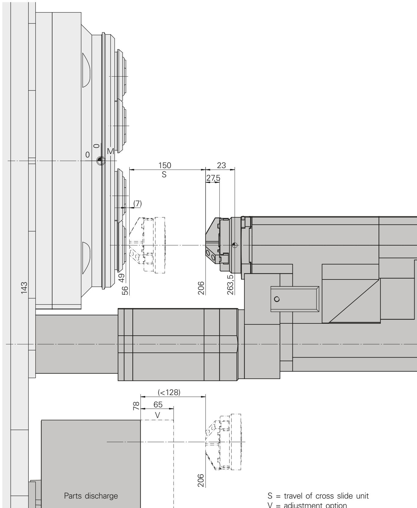
**Synchronized spindle INDEX MS40-8****Rear end machining on swivel axis 7.2, 8.1****Rear end machining unit on cross slide unit 7.1, 8.2, 7.3/8.3, 7.4/8.4**
