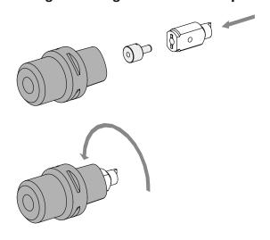
For removal, the socket wrench must be turned through 180°.
