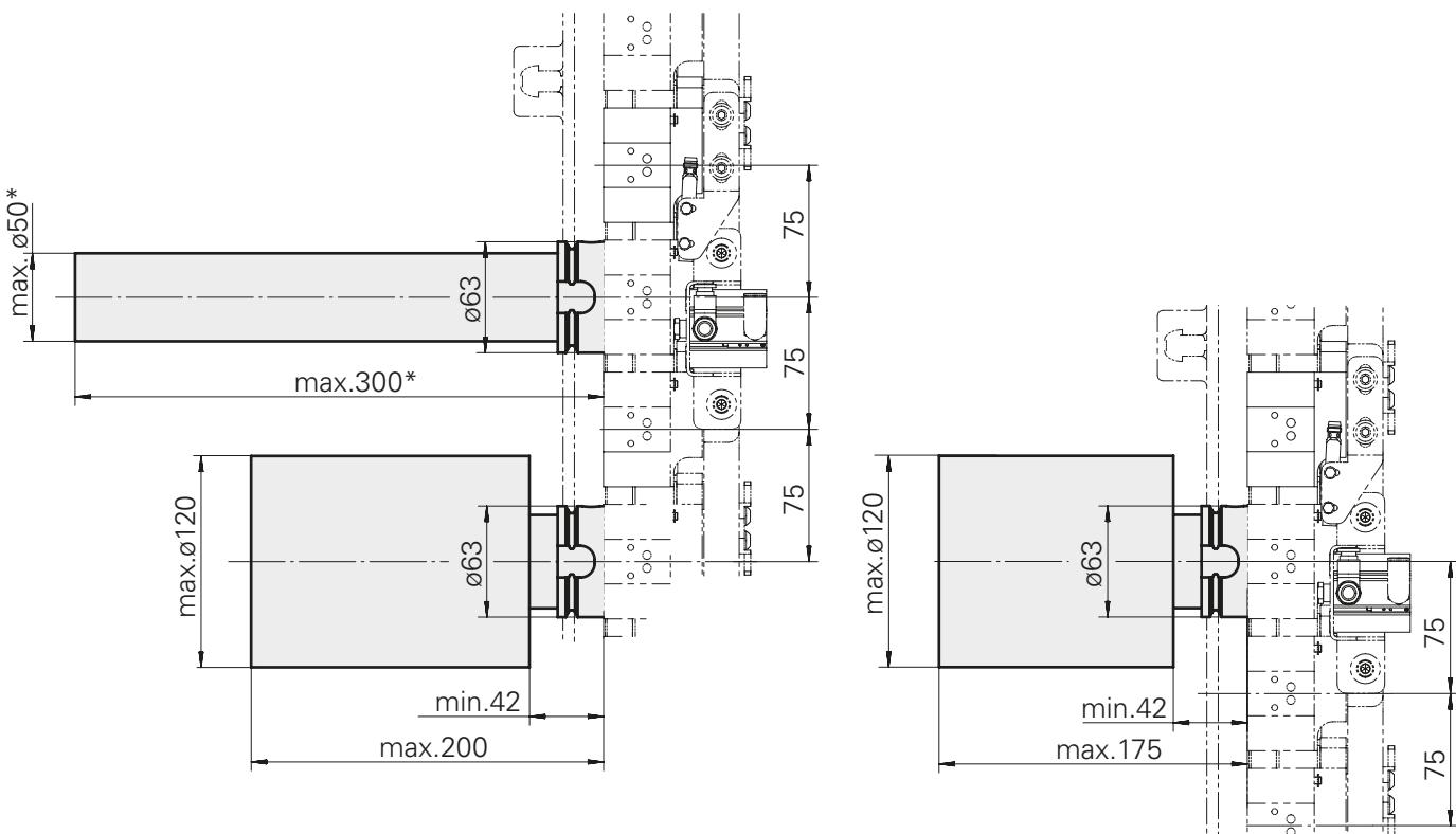
\* = Special tool change cycle for tool L = 200 to 300 mm
