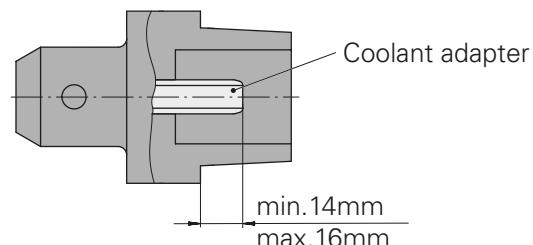
**Coolant adapter set and socket wrench**
