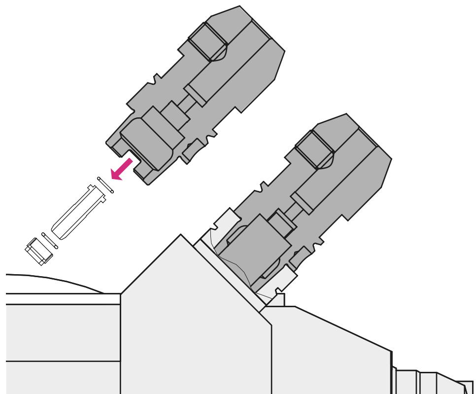
**Upper tool carrier, with motorized milling spindle****1 live tool station HSK63**
