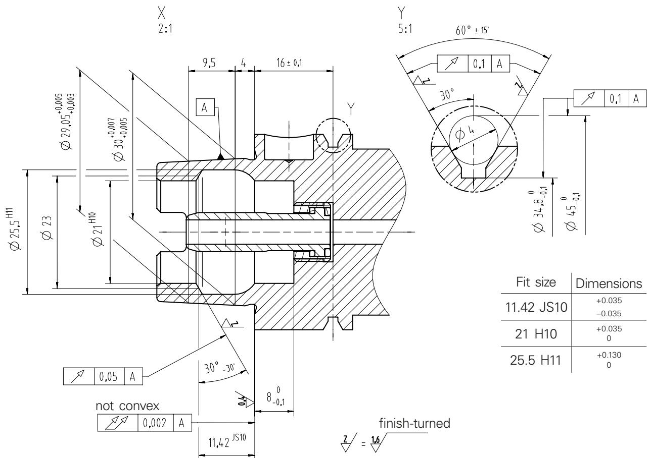
**HSK tool dimensions HSK40 A****Tool magazine 1**
