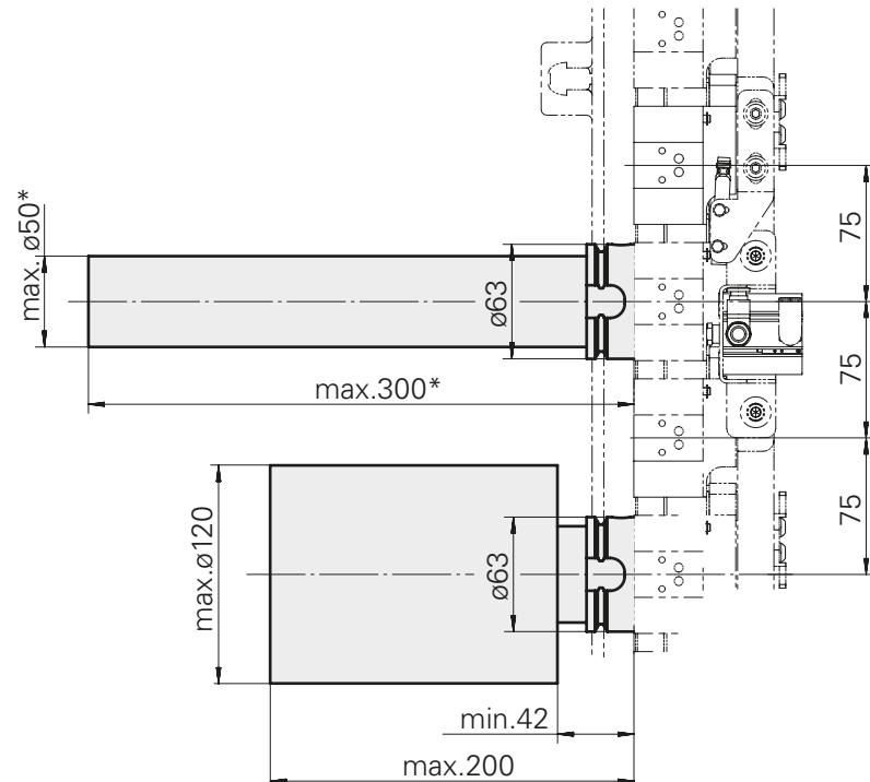
\* = Special tool change cycle for tool L = 200 to 300 mm
