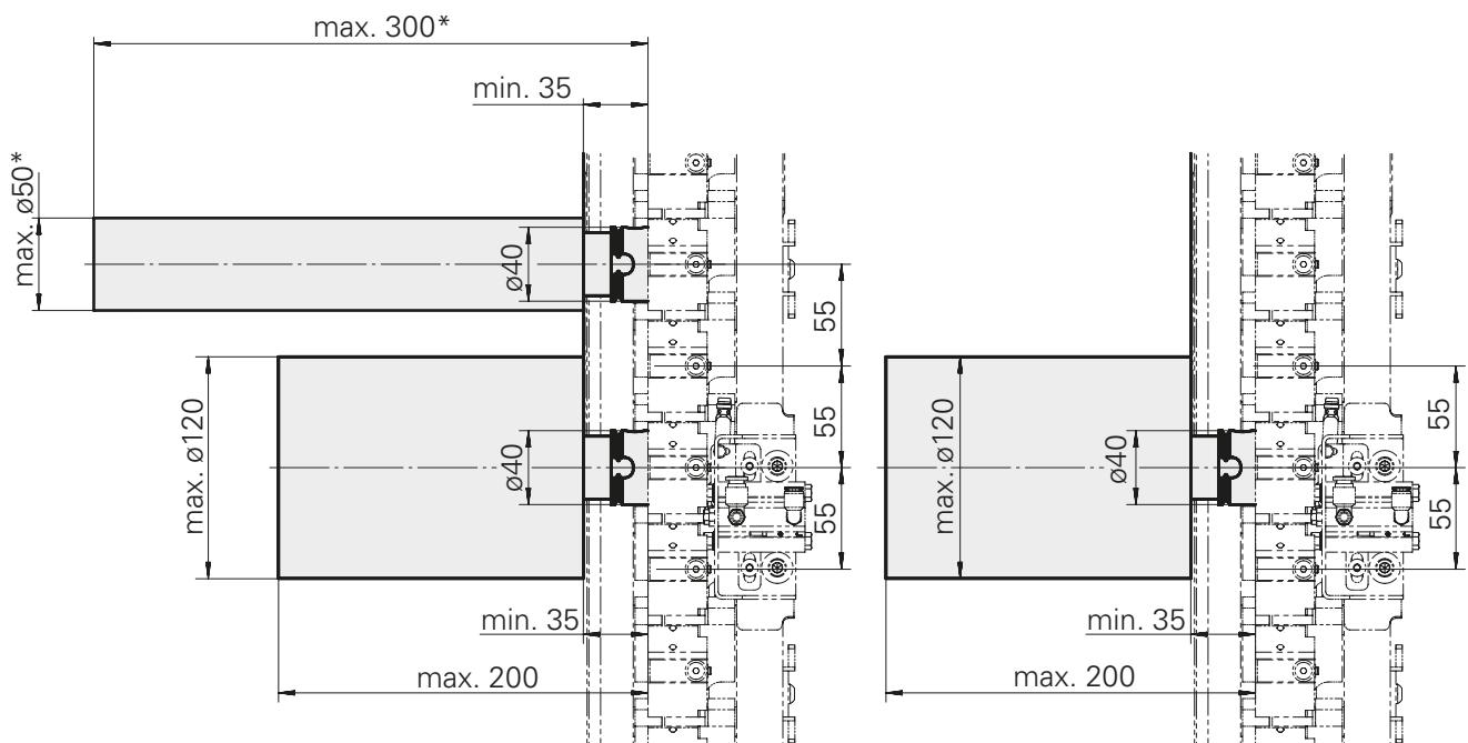
\* = Special tool change cycle for tool L = 200 to 300 mm
