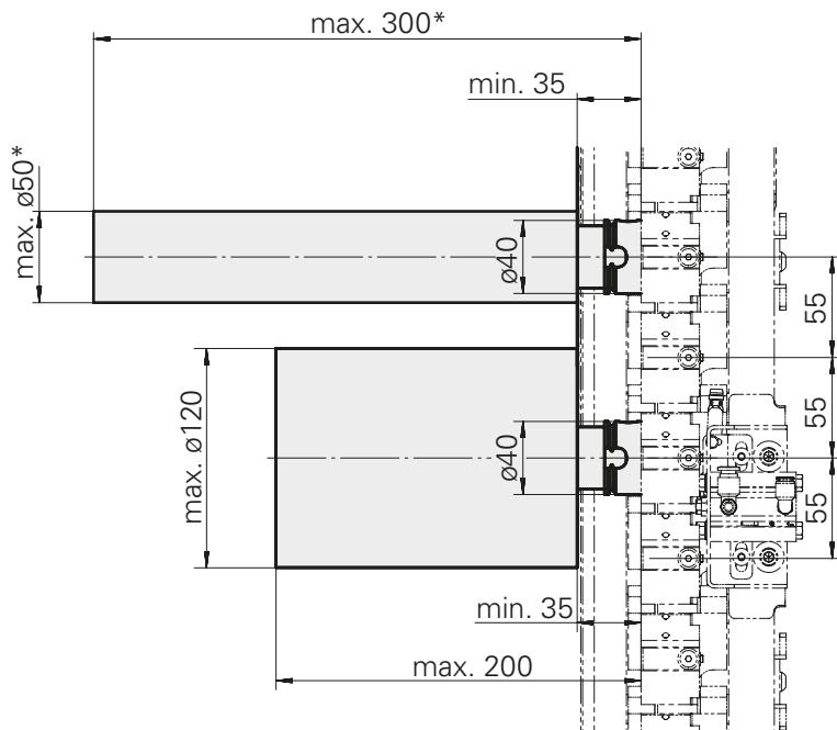
\* = Special tool change cycle for tool L = 200 to 300 mm
