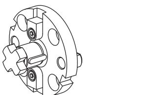
**10670447 Milling cutter holding block**
