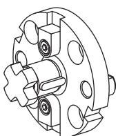
**10670447 Milling cutter holding block**
