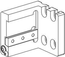
**10804363 Grooving tool holding block, vertically adjustable**
