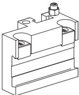
**10410270 Grooving tool holding block, vertically adjustable**
