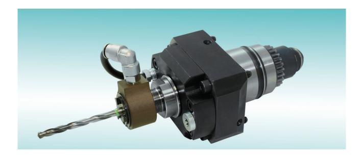
Convert live INDEX TRAUB tool holders from external cooling to internal cooling in just two minutes.
