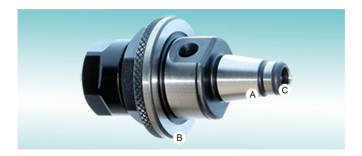
The Quick-Change System WFB combines the precision of a conventional tool holder with the flexibility of a modular tool holder system in an impressive way. The patented combination of a cone (A) with a front-end contact face (B) provides enormous stability and exceptionally high change accuracy. An additional support ring (C) reduces any lateral forces to a minimum.
