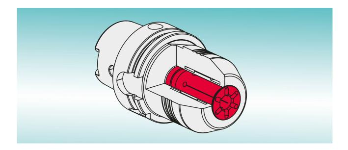
Besides fine machining operations such as reaming or threading, the robust HSK hydraulic expansion chucks can also be used for heavy-duty volume cutting.
