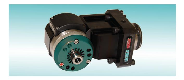
The fluid spindle, established in the industry for many years, is now being replaced by a new, optimized successor version. The new spindle allows you to cover the entire speed range up to 55,000 rpm. A new locking mechanism also simplifies tool clamping.
