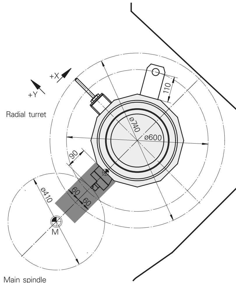
**Work area****INDEX B500** from machine No. 12010119, **TRAUB TNA500.2** from machine No. 12020123**Radial turret VDI40, Counter spindle**
