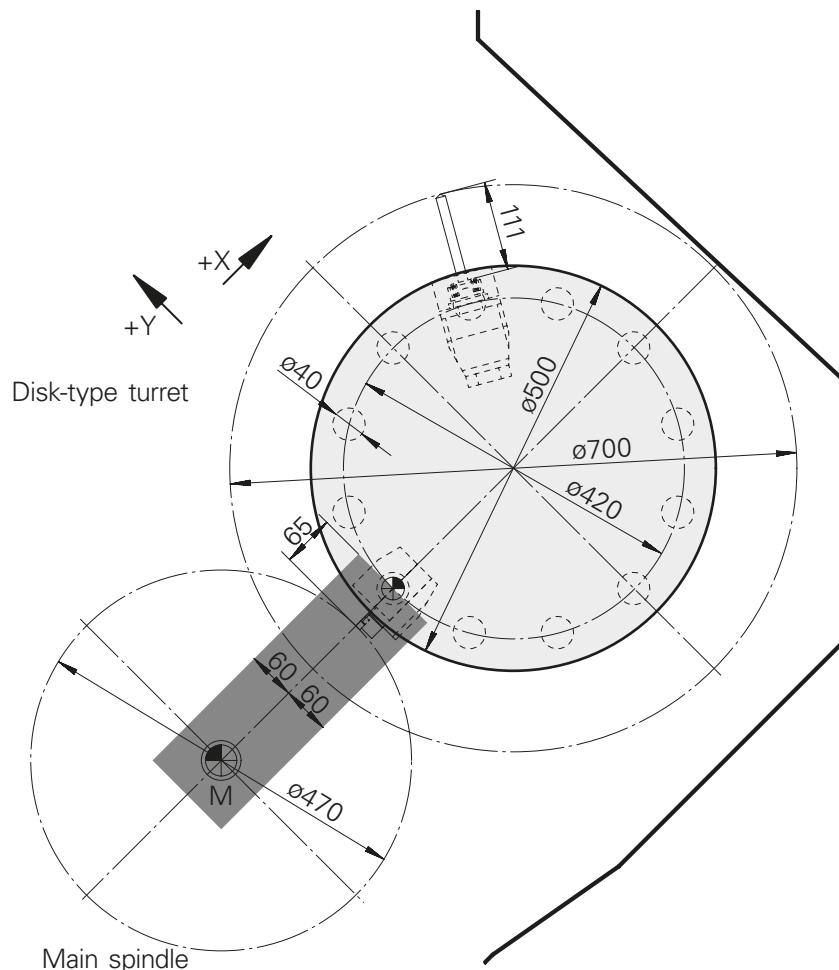
**Swivel range of INDEX B500, TRAUB TNA500.2****Radial turret with tooling system VDI40**
