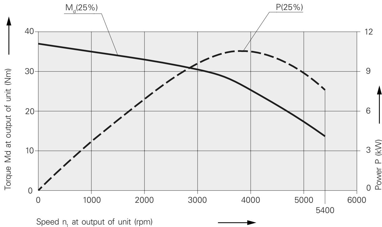
**Performance diagram valid for TRAUB TNA500.2****Live tools VDI40, Radial turret and Disk-type turret**
