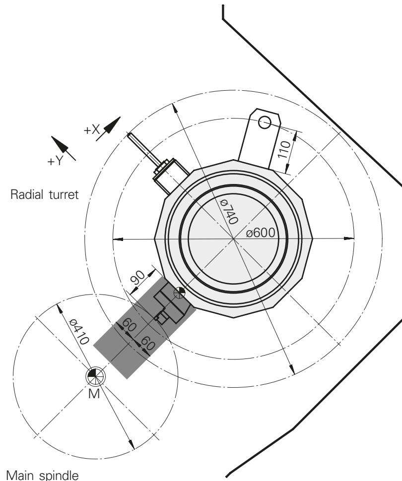
**Work area****INDEX B500** from machine No. 12010119, **TRAUB TNA500.2** from machine No. 12020123**Disk-type turret VDI40, NC tailstock**
