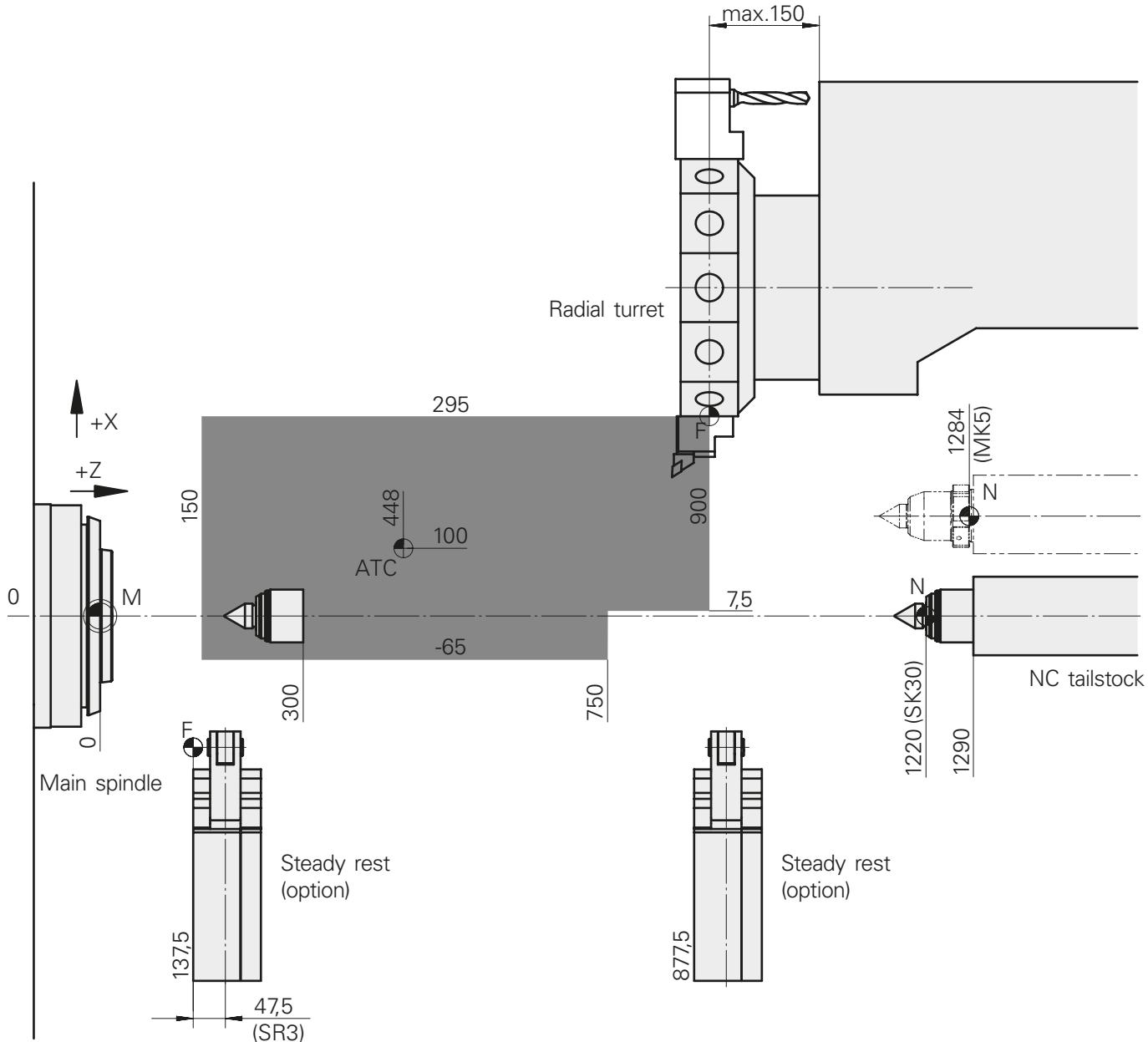
**Work area****INDEX B500** from machine No. 12010119, **TRAUB TNA500.2** from machine No. 12020123**Radial turret VDI40, NC tailstock**
