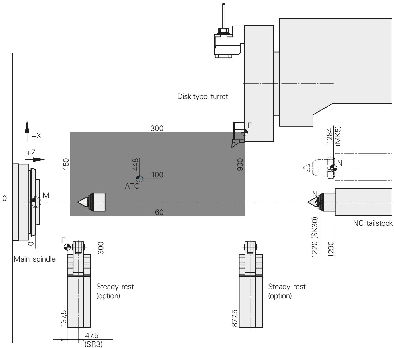
**Work area****INDEX B500** from machine No. 12010119, **TRAUB TNA500.2** from machine No. 12020123**Disk-type turret VDI40, NC tailstock**
