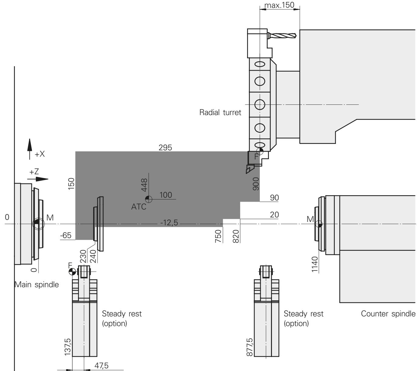
**Work area****INDEX B500** from machine No. 12010119, **TRAUB TNA500.2** from machine No. 12020123**Radial turret VDI40, Counter spindle**
