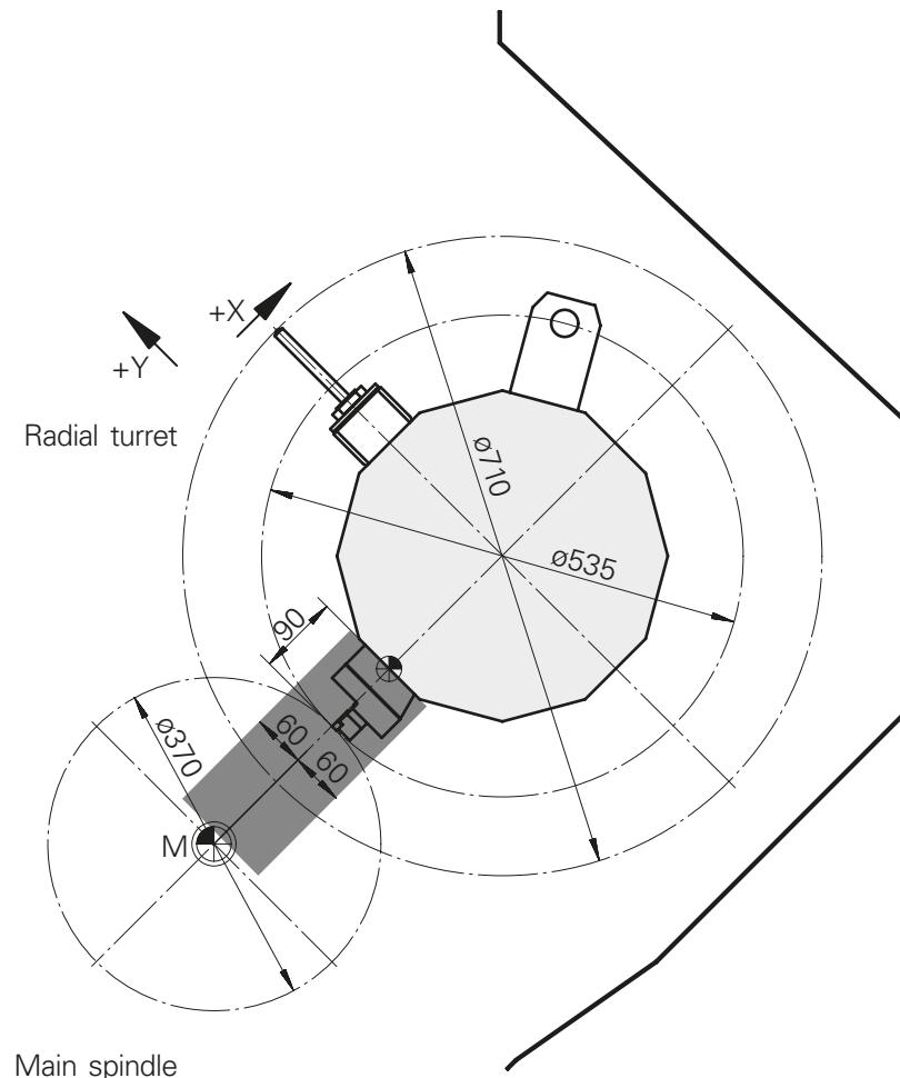
**Work area****INDEX B400** from machine No. 12010119, **TRAUB TNA400.2** from machine No. 12020123**Radial turret VDI40, NC tailstock**
