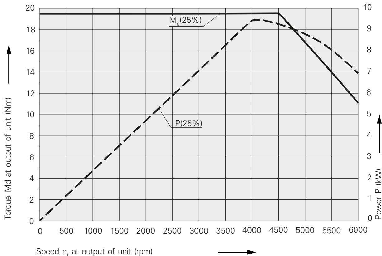
**Performance diagram valid for TRAUB TNA400.2****Live tools VDI40, Radial turret and Disk-type turret**
