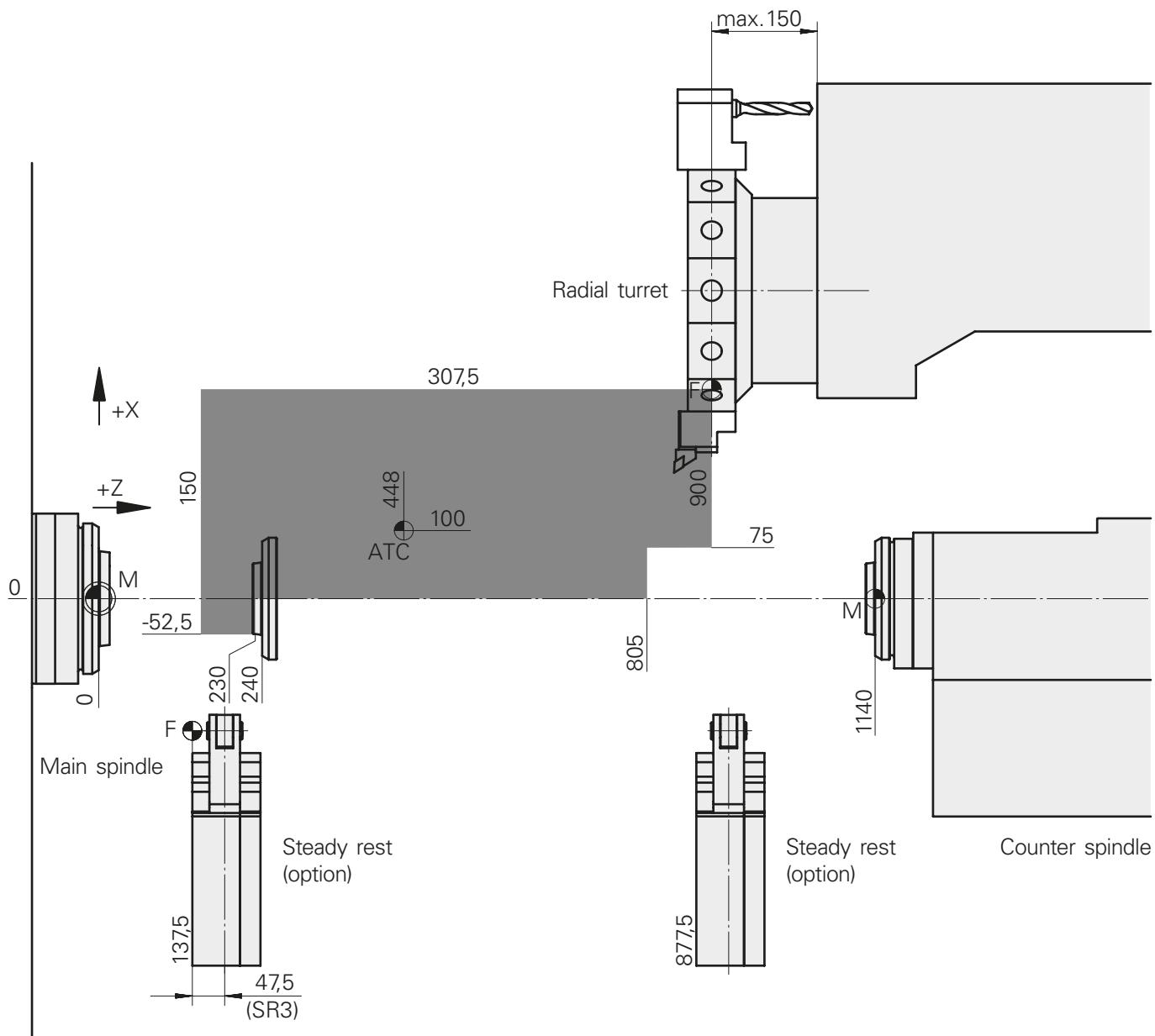
**Work area****INDEX B400** from machine No. 12010119, **TRAUB TNA400.2** from machine No. 12020123**Radial turret VDI30, Counter spindle**
