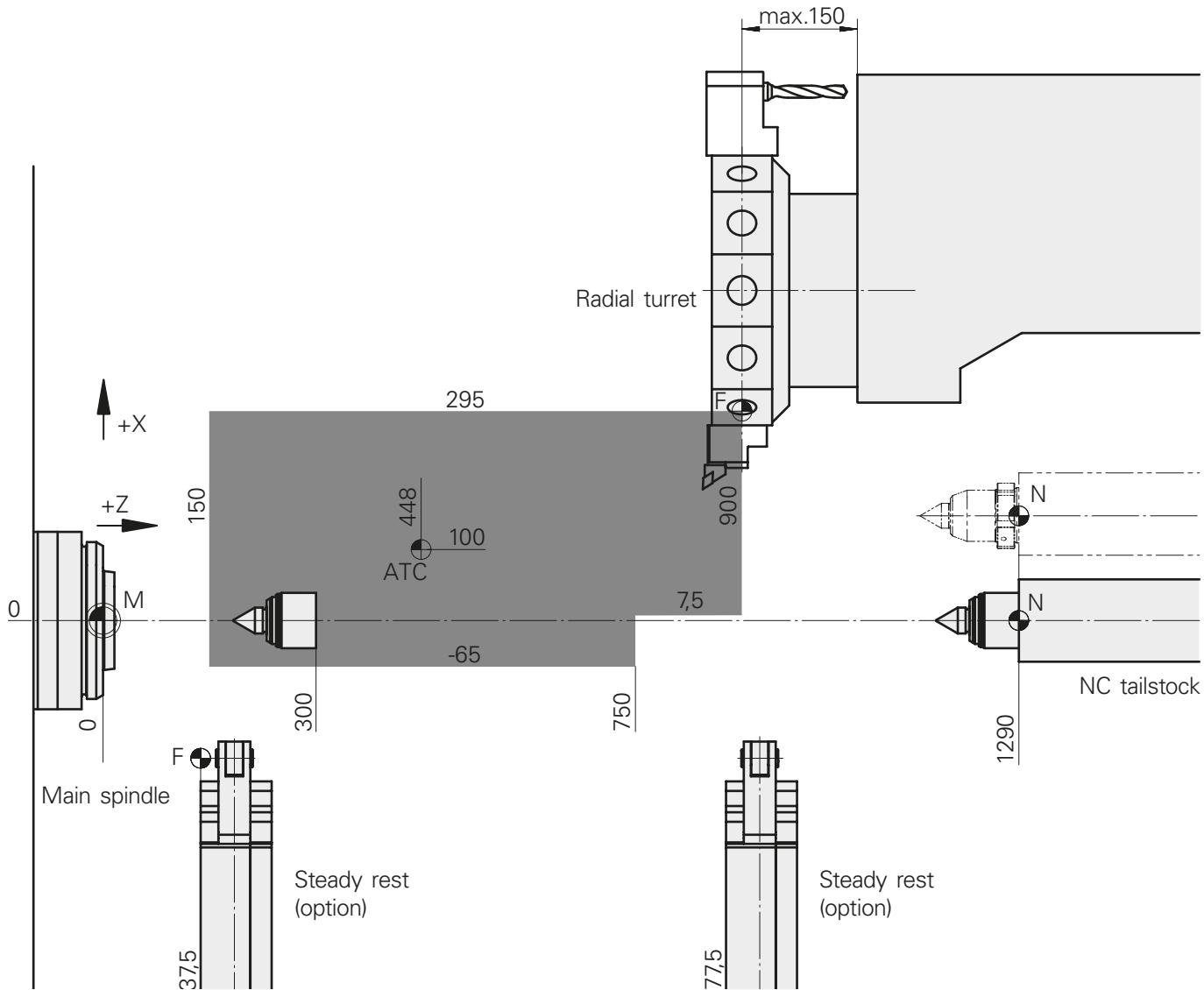
**Work area****INDEX B400** from machine No. 12010119, **TRAUB TNA400.2** from machine No. 12020123**Radial turret VDI40, NC tailstock**
