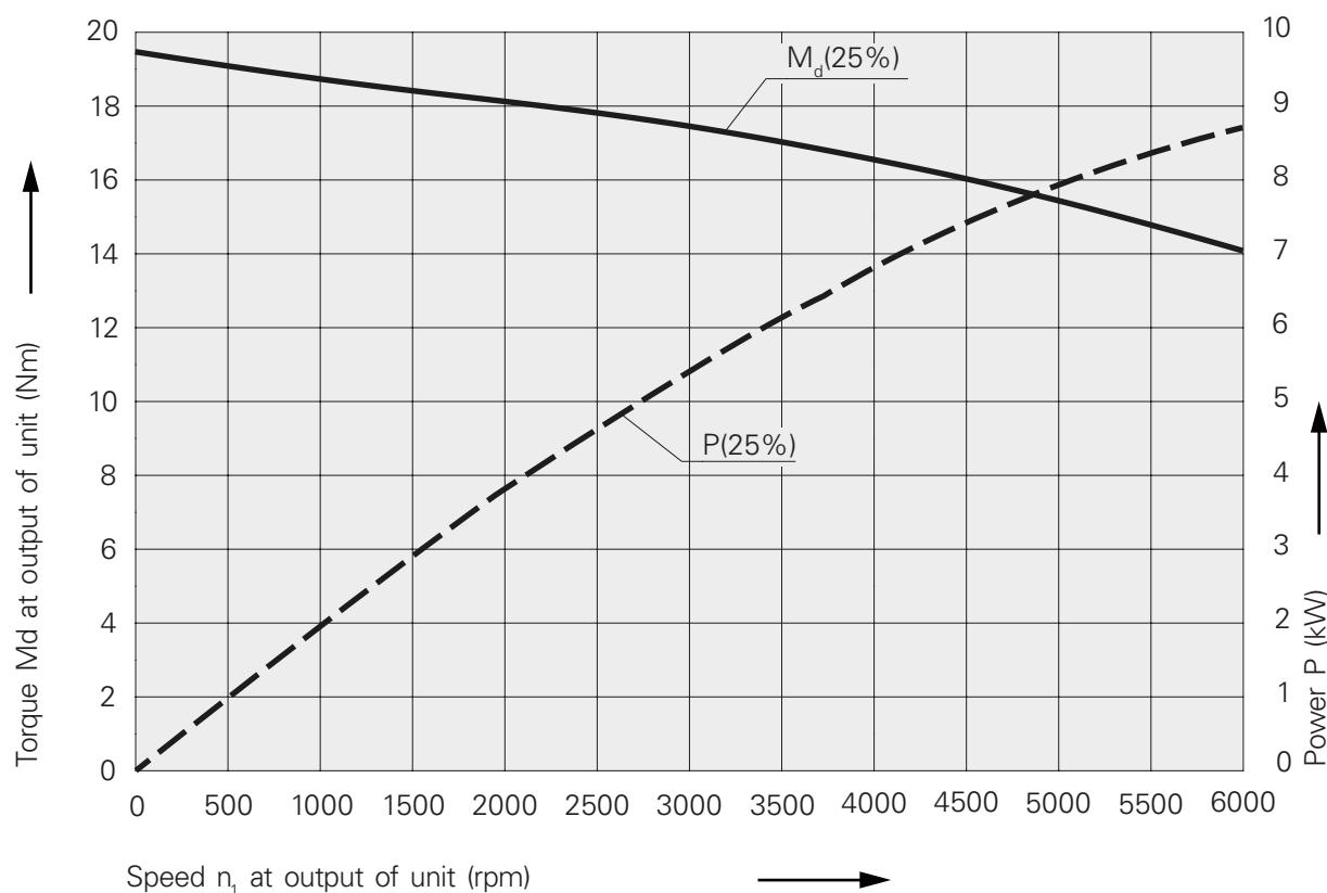
**Performance diagram valid for INDEX B400****Live tools VDI40, Radial turret and Disk-type turret**
