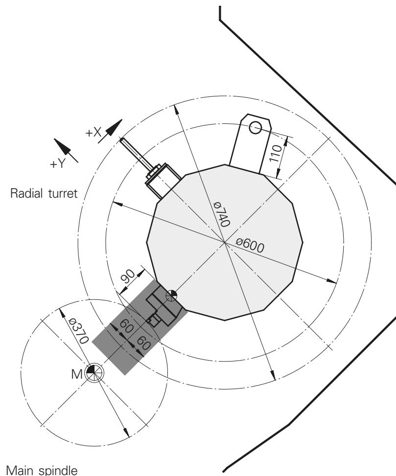
**Work area****INDEX B400** from machine No. 12010119, **TRAUB TNA400.2** from machine No. 12020123**Radial turret VDI40, Counter spindle**
