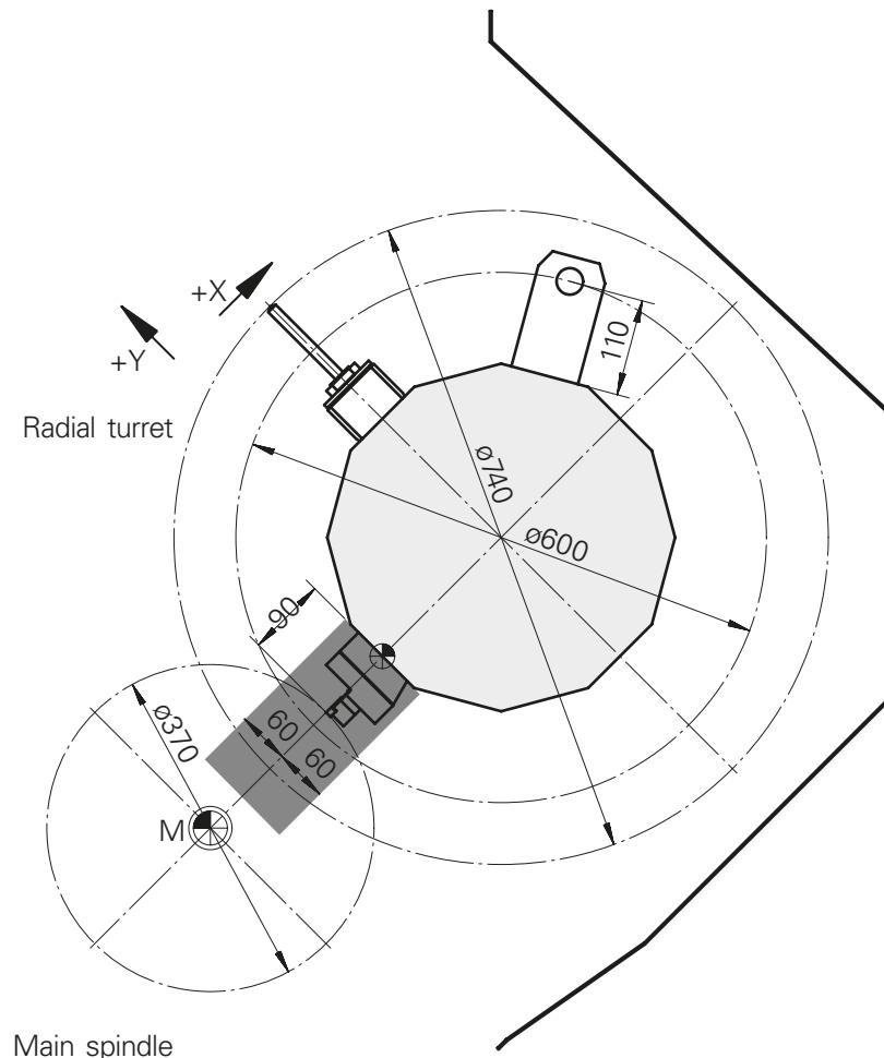
**Work area****INDEX B400** from machine No. 12010119, **TRAUB TNA400.2** from machine No. 12020123**Disk-type turret VDI40, NC tailstock**
