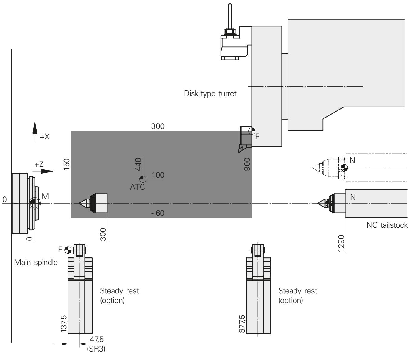
**Work area****INDEX B400** from machine No. 12010119, **TRAUB TNA400.2** from machine No. 12020123**Disk-type turret VDI40, NC tailstock**
