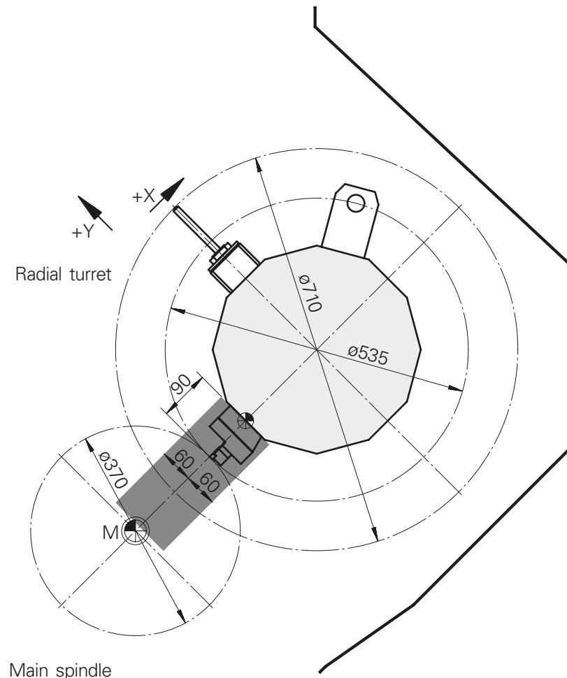
**Work area****INDEX B400** from machine No. 12010119, **TRAUB TNA400.2** from machine No. 12020123**Radial turret VDI30, Counter spindle**
