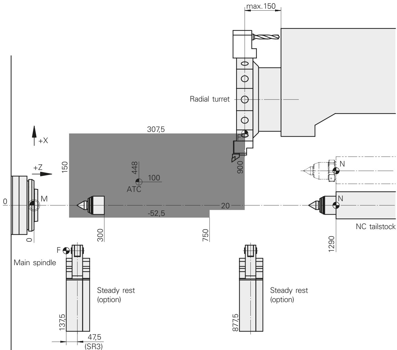
**Work area****INDEX B400** from machine No. 12010119, **TRAUB TNA400.2** from machine No. 12020123**Radial turret VDI30, NC tailstock**
