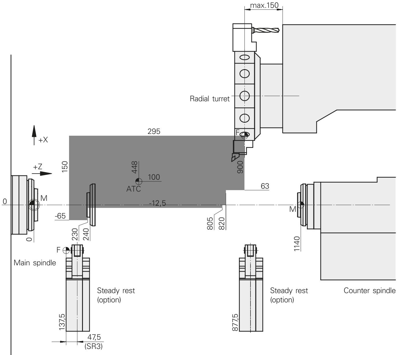
**Work area****INDEX B400** from machine No. 12010119, **TRAUB TNA400.2** from machine No. 12020123**Radial turret VDI40, Counter spindle**
