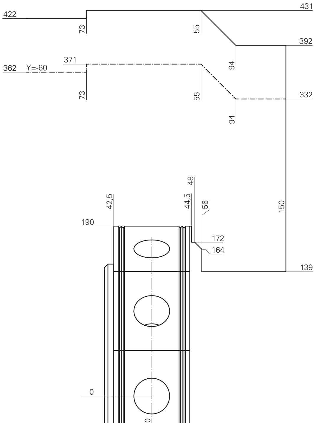
**Swivel range INDEX B400, TRAUB TNA400.2****Disk-type turret with tooling system VDI40**
