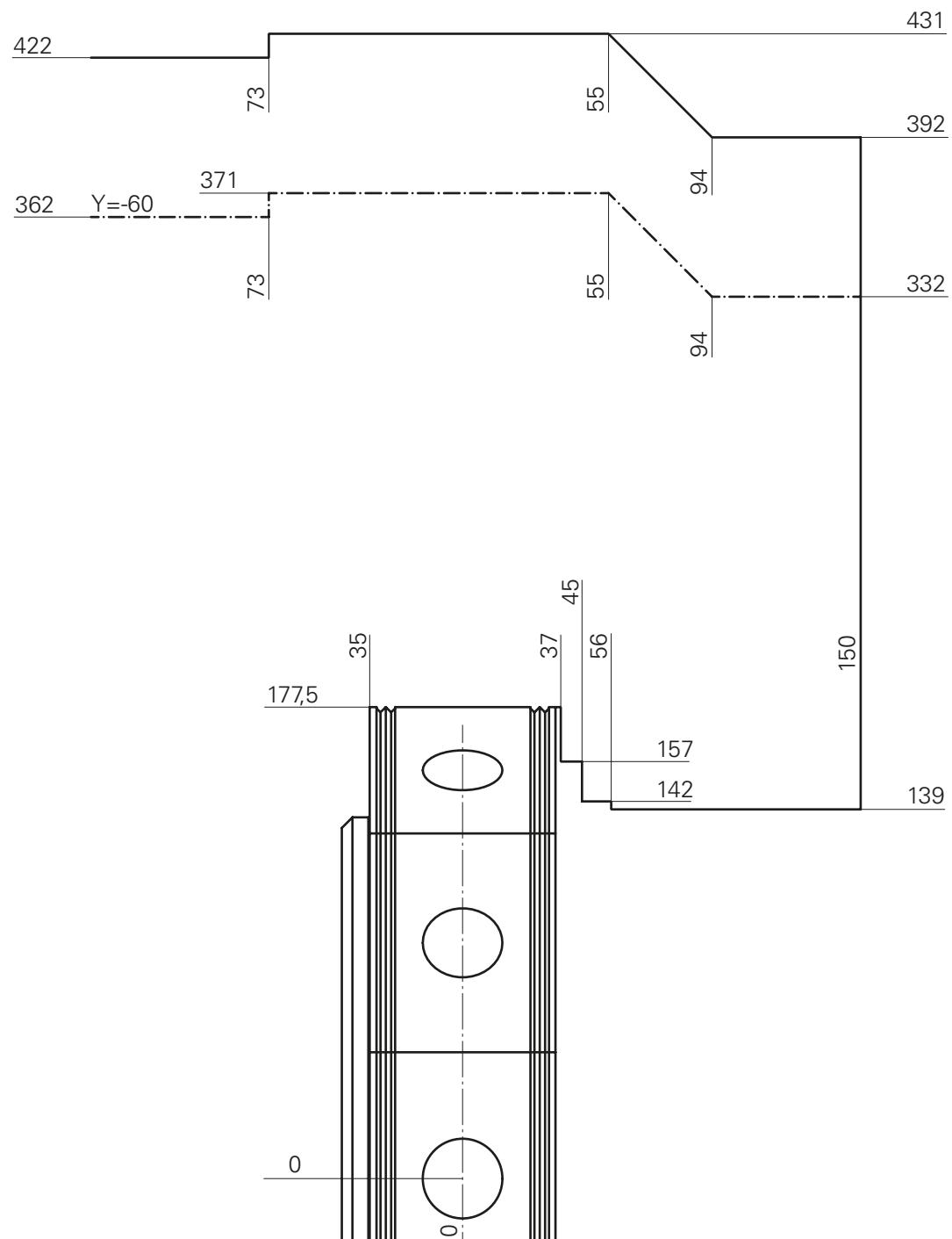
**Swivel range INDEX B400, TRAUB TNA400.2****Radial turret with tooling system VDI40**
