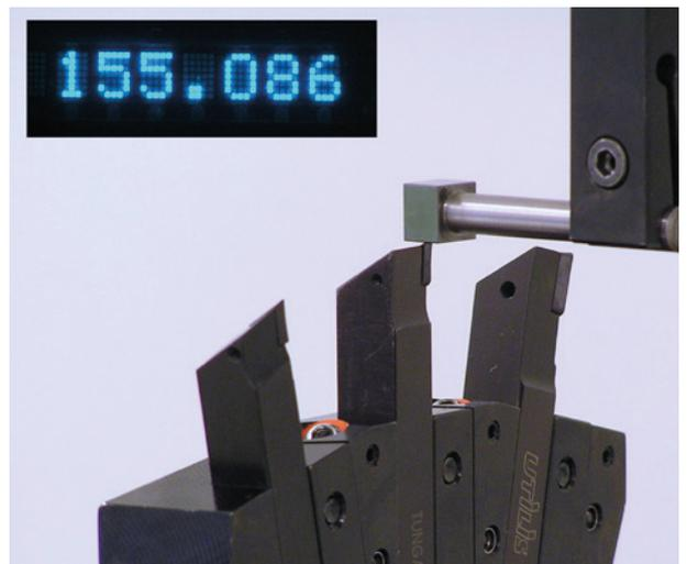
The measured value is a radius value; 40 mm must be subtracted for 11008063 (75 mm for 10826369), for entering into the tool memory, this value must be doubled
