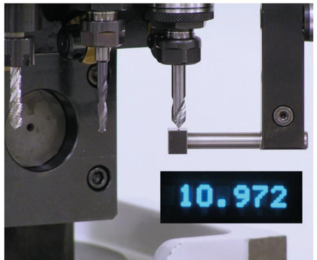
Tool holders with machining towards the main spindle partially cannot be measured in the correct installation position. In this case, the sign of the measured value must be inverted: + becomes - and - becomes +.
