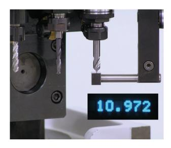
Tool holders with machining towards the main spindle partially cannot be measured in the correct installation position. In this case, the sign of the measured value must be inversed: + becomes - and - becomes +.
