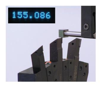
The measured value is a radius value; 40 mm must be subtracted for 11008063 (75 mm for 10826369), for entering into the tool memory, this value must be doubled
