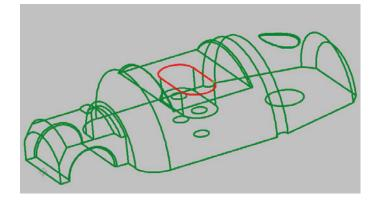
The individual geometry elements can then be selected and projected into the geometry editor as 2D contours. The position before the projection is essential. The function connects contiguous geometry elements to a contour. If elements are selected that have no connection, several contours will be displayed in the geometry processor after the projection. These "2D contours" can be saved in the geometry processor and reloaded during editing operations.
